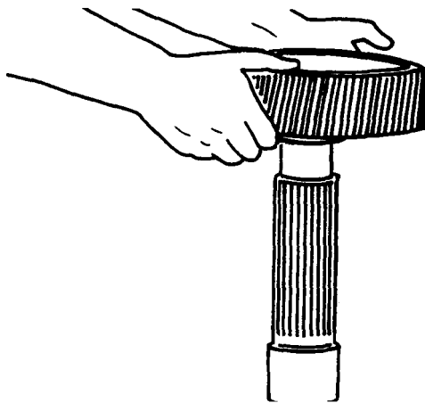
4. Remove the large idler gear.
