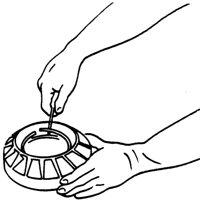
9. Remove the reaction member and freewheeling assembly.
