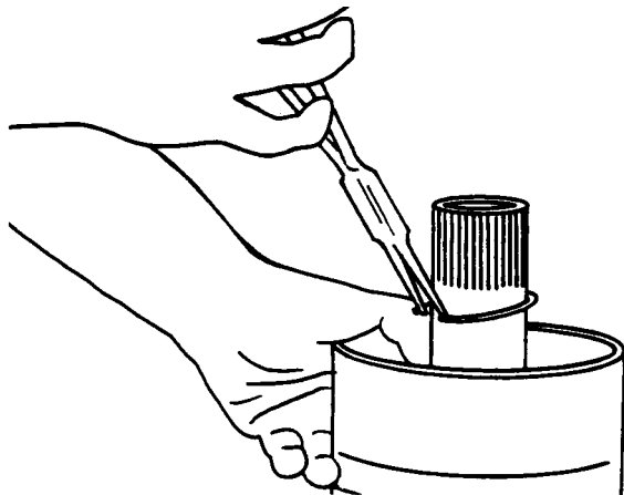
11. Remove the return spring retainer ring.
