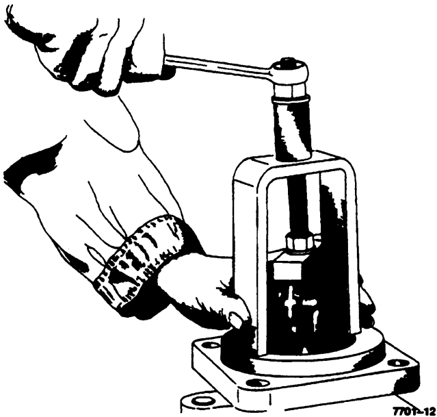
12. Use a bearing puller to remove the outboard bearing.
