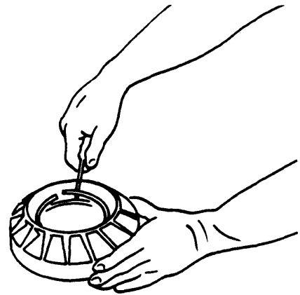
12. Install the outer race to reaction member retainer ring.
