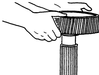
2. Position the large idler gear on the shaft with the long hub on the gear down.
