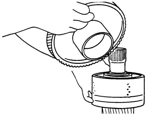
15. Install the low clutch driven gear and the hub into the clutch drum. Align the splines on the clutch hub with the internal teeth of all the friction discs.
